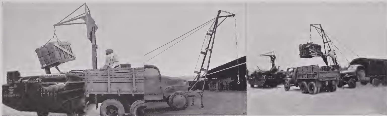
FIGURE 59. Transfer rig arrangements used to transfer cargo from DUKWs to trucks in Normandy landings.
